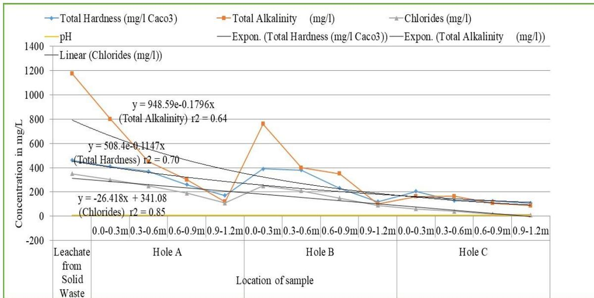
Figure 3: Variation of Total Hardness, Total Alkalinity, Chloride and pH with Depth
